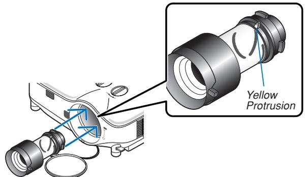
2. **Rotate the lens clockwise.**
