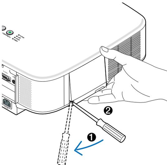
2. Loosen the two screws securing the lamp housing until the phillips screwdriver goes into a freewheeling condition. The two screws are not removable. Remove the lamp housing by holding it.
